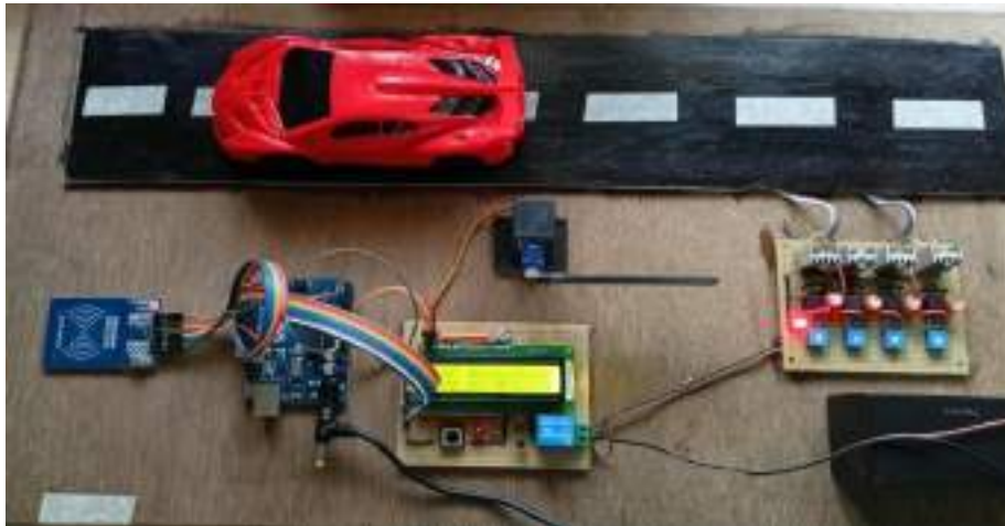
Figure 2: RFID Based Automatic Toll Collection System for Dynamic Charging Vehicles
