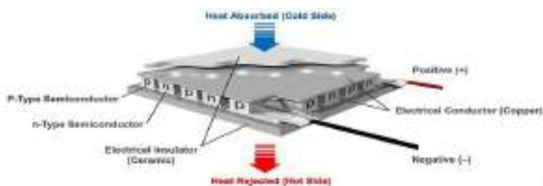
Figure 1: Diagram of a typical thermoelectric couple
